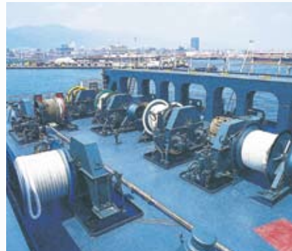
●系泊绞车 Mooring winch
