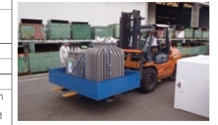
Transport of transformers taken out of service (PCBs are used in the insulation oil)
